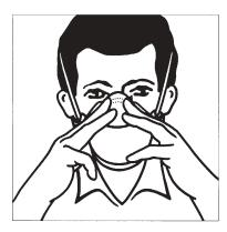
5. Using both hands, mould noseclip to the lower part of the nose.
