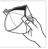
1. The noseclip is located in the top panel. Pre-form the noseclip by gently bending at the centre of the panel. Hold the respirator in one hand and pull out the bottom panel to form a cup.
